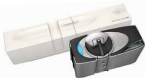
The Malvern Mastersizer 2000 (pictured top), is a renowned instrument for measuring particle size.
