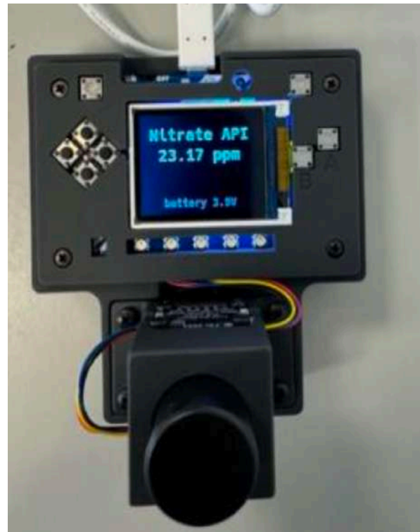
Open-source colorimeter used in Charlie's research
